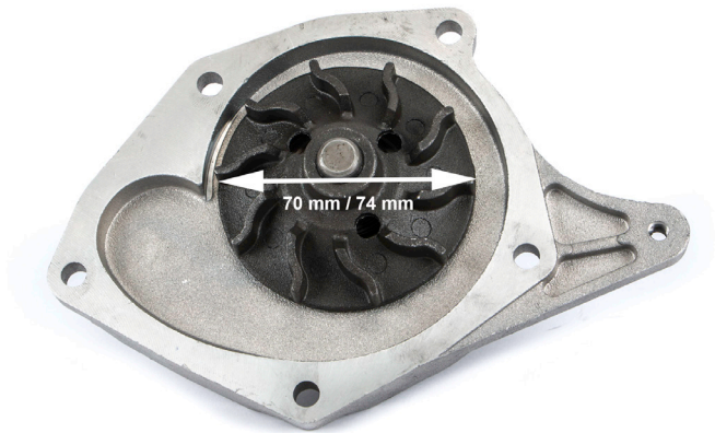
Determining the impeller diameter after removal of the coolant pump
