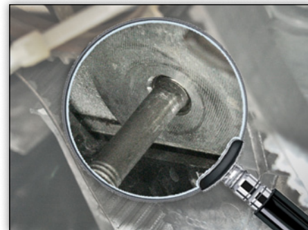
Image 2: The stud is correctly screwed in.
